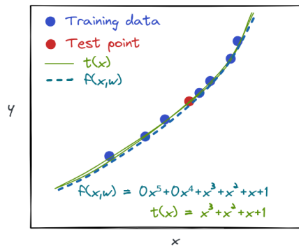
Figure 5: If there was no noise, a too-complex model class wouldn't necessarily be a problem.
