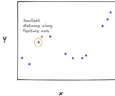
Figure 1: The nearest neighbor to the orange test point is the one that has the smallest distance in the feature space.
